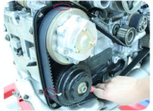
Picture 8: Align timing marks
