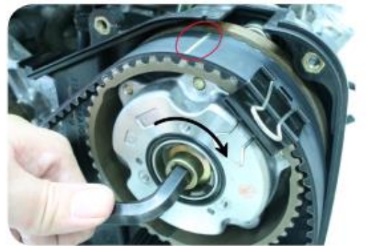
Picture 9: Secure belt by clip and align timing mark
