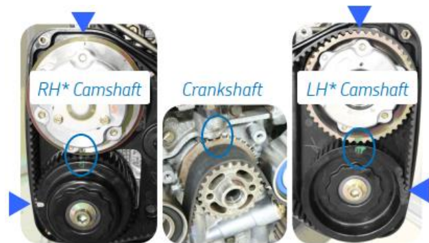
Picture 2: Camshafts and Crankshaft at correct alignment. *RH/LH Camshaft orientation according to OE service manual.
