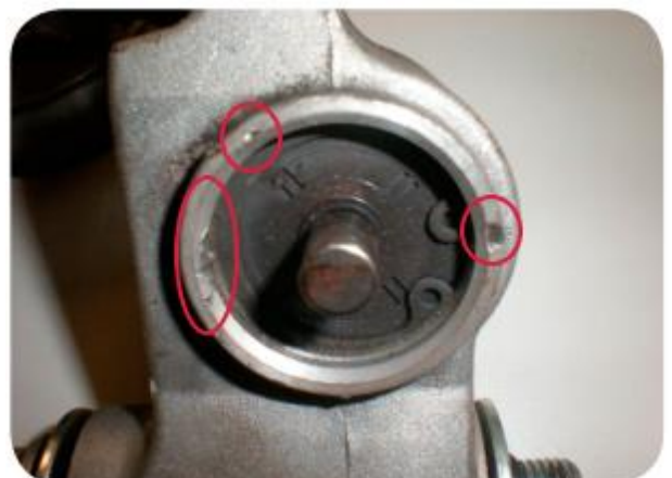
Picture 7: Dent marks on the tensioner body
