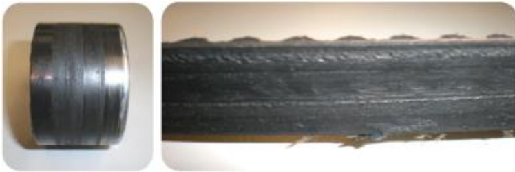
Picture 12: Overheated marks
